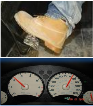
Step 4 (b) Keep accelerating the engine by pressing the gas pedal at RPM between 2k-3K.
